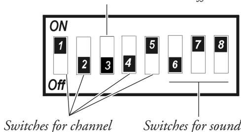
The smoke detector is equipped with a transmitter that sends signals wirelessly to the receiver installed in the Lynx system. The transmitter is located under the cover and has an 8-pole microswitch that is used for two purposes:
