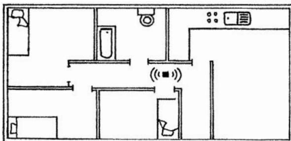
Because smoke rises, and to ensure that the smoke detector is activated as rapidly as possible in the event of fire, it should be located in the ceiling at least 50 cm from a wall. If ceiling mounting is not possible, it should be located near the top of a wall. If the ceiling is sloping, it should be mounted about 90 cm from the highest point.
